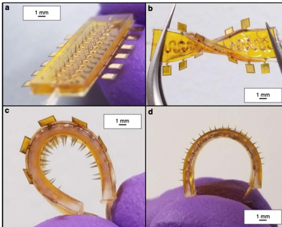
**Figure 3.** Optical image of microserpentine sensor device. The image is reproduced with permission from [5]
