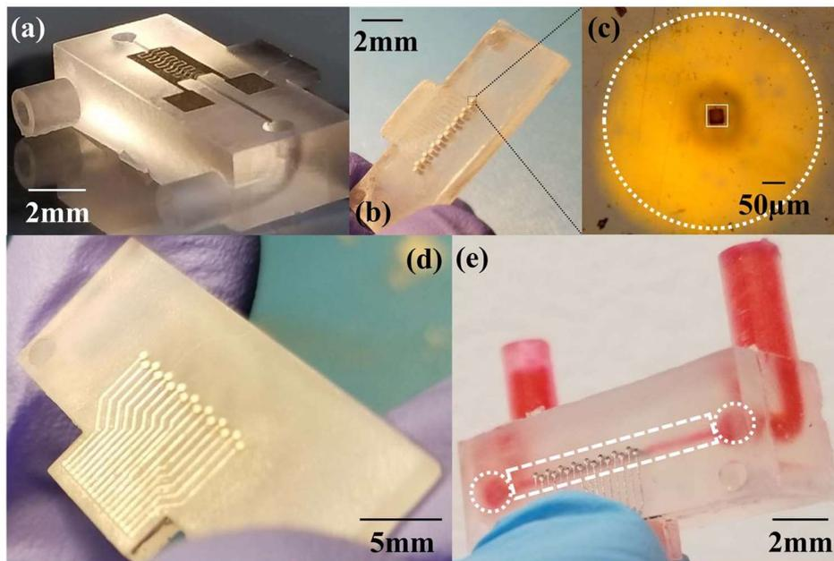
**Figure 2.** Optical micrograph of the biosensor using MEAs and IDEs. The image is reproduced with permission from [4]
