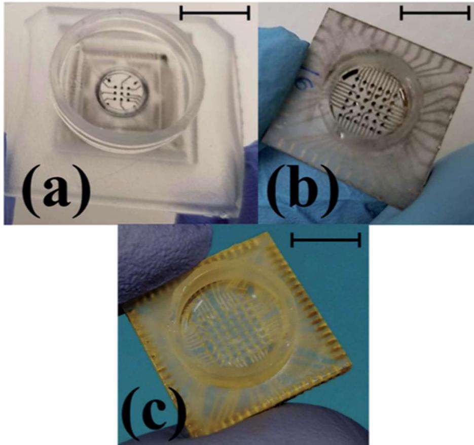
**Figure 1.** Optical images of different culture wells with 3x3, 6x6 and 8x8 MEAs. 10 mm scale bar. The image is reproduced with permission from [3]. Gold or platinum features are used in the microelectrodes to transport electrical signals with minimal restriction to the flow of electrical current and because of the biocompatibility of these materials [3]. Electrogenic cells can be monitored by using this MEAs, which can record and send electrical signals to the cell network.
